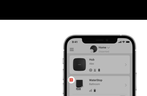
If a malfunction is detected in WaterStop (for example, there is no connection with the hub or range extender), the malfunction counter is displayed in the device field in Ajax app.
