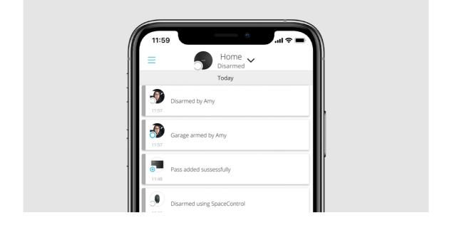
When a Tag or Pass is linked to a user, it fully inherits the rights to manage the user's security modes. For example, if a user was able to manage only one group, then the bound Tag or Pass will have the right to manage only this group.
