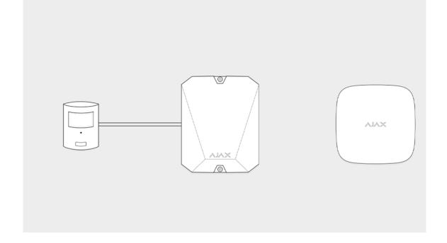
MultiTransmitter can be used to connect panic and medical alarm buttons, indoor and outdoor motion detectors, as well as detectors tracking opening, vibration, breaking, fire, gas, leakage, etc. The type of device is indicated in the zone settings. The text of notifications about alarms and events of the connected device, as well as event codes transmitted to the Central Monitoring Station (CMS) of the security company depend on the selected device type.
