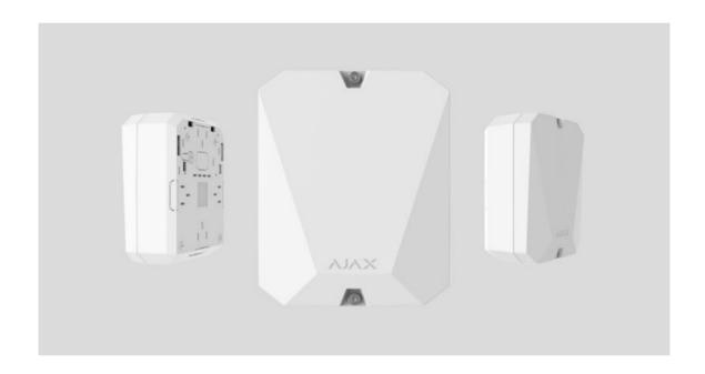
**MultiTransmitter** is an integration module with 18 wired zones for connecting third-party detectors to the Ajax security system. To protect against dismantling, MultiTransmitter is equipped with two tampers. It is powered from the mains 100–240 V AC, and can also run on a 12 V backup battery. It can supply 12 V power to connected detectors.
