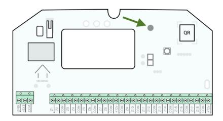
MultiTransmitter LED indicator may light up white, red, or green, depending on the status of the device. Please note that the LED indicator is not visible when the body lid is closed, but the status of the device can be found in the Ajax app.
