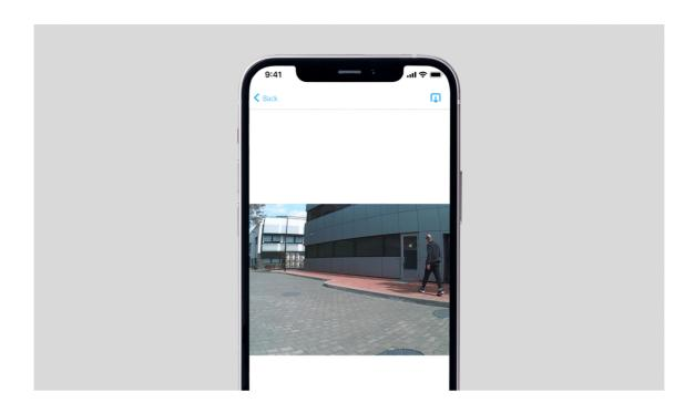
When the detector is triggered, the built-in MotionCam Outdoor camera can take 1 to 5 images with a resolution of 320 × 176 and up to 3 images with a resolution of 640 × 352 pixels. The detector has infrared illumination for shooting in the dark, which is activated only when an alarm is raised.
