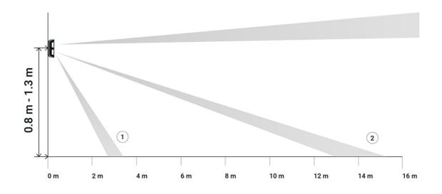
The detection distance is adjusted using the **Detection Distance** scrollbar on the rear panel of the detector. When choosing the installation location, consider the maximum detection range of the detector. It depends on the sensitivity, the position of the Detection Distance scrollbar, the type and speed of the person's movement (running, walking), and the ambient temperature.
