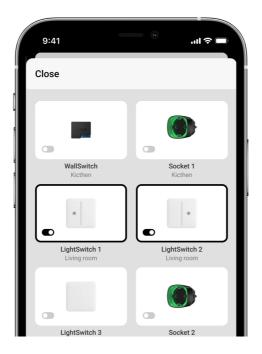
The lighting also can be controlled in the **Control** • menu. To do this, go to the **Control** • menu and swipe up. All control devices added to the hub will appear in the list. Click on the switch in the **LightSwitch** field, and the state of the device's contacts will change to the opposite. The lighting will switch on or off.
