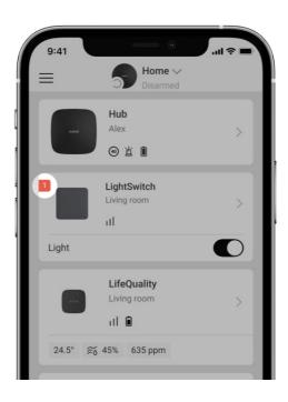
When a device identifies a fault (for example, there is no connection with the hub), the Ajax app displays a fault counter in the device field.
