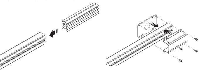
Fix the boom to the anchoring plate.
