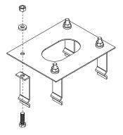
Fit the anchoring plate in the iron cage.
