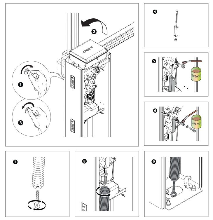
Lubricate the spring when it is fully extended.
