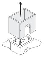
Fill the hole with soil around the concrete block. Remove the nuts from the screws.
