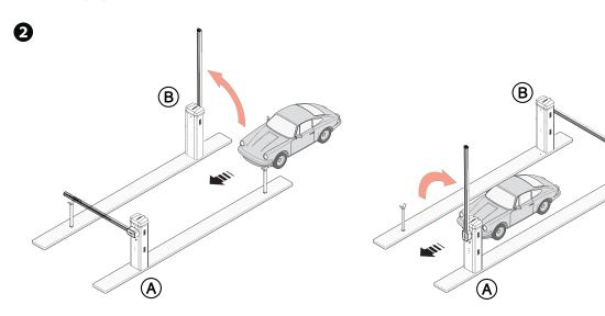
3 OPEN-CLOSE command (2-7) on barrier A or B for emergency opening
