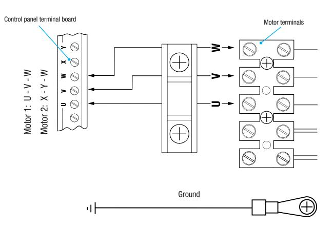
F If only using one motor, such as with one-leaf gates, connect it to W X Y (M2) regardless of which side it is installed on.
