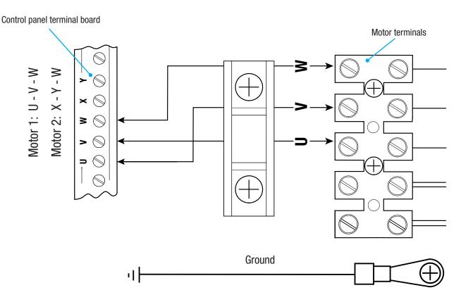
Figure 1 only using one motor, such as with one-leaf gates, connect it to W X Y (M2) regardless of which side it is installed on.
