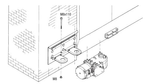
Join and secure the two arms using the washer and M8x16 screw. Release the motor (see p. 7) and secure the curved semi-arm to the "A" bracket using the M12X50 screw and the M12 nut making sure it runs freely. For right-hand application see fig. 2.
