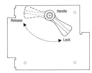
In the event of power outages or breakdowns, release the gearmotor using the apposite handle.
