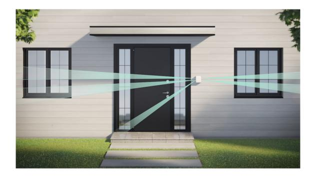
DualCurtain Outdoor is suitable for the protection of the area around the secured site. It allows to guard the perimeter, leaving space for free movement inside. The detector can be installed both outdoors and indoors.
