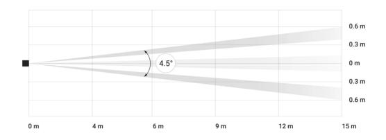
Horizontal viewing angle of the detector
